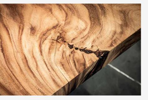
A detailed study is performing on every slab in order to decide how knots, splits and checks are to be dealt with. Thus ensuring the final results is aesthetically pleasing.
